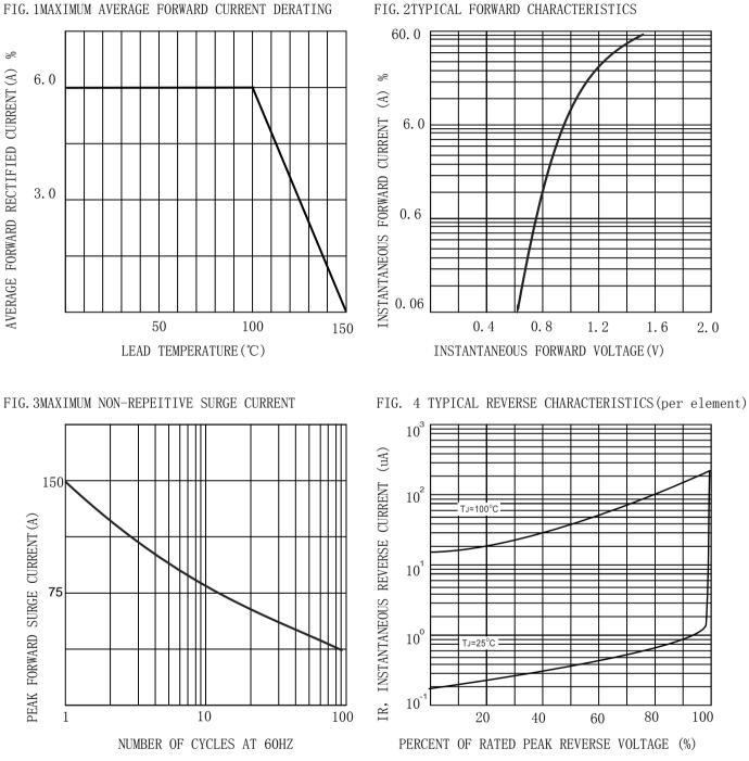
FIG. 1MAXIMUM AVERAGE FORWARD CURRENT DERATING
